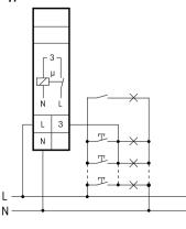
3-wire circuit with attic lighting, not resettable.
