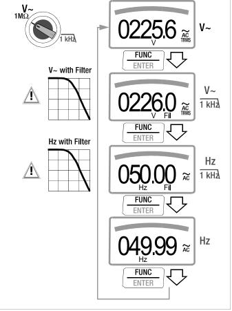
5.1.3 Alternating Voltage and Frequency Measurement V AC and Hz with Selectable Low-Pass Filter (METRAHIT X-TRA OUTDOOR TECH | PRO only)
