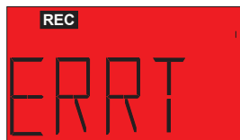
Figure 1: Error in the connection of the earth leakage transformer.
