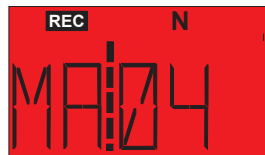
Figure 11: Screen after a circuit breaker trip.
